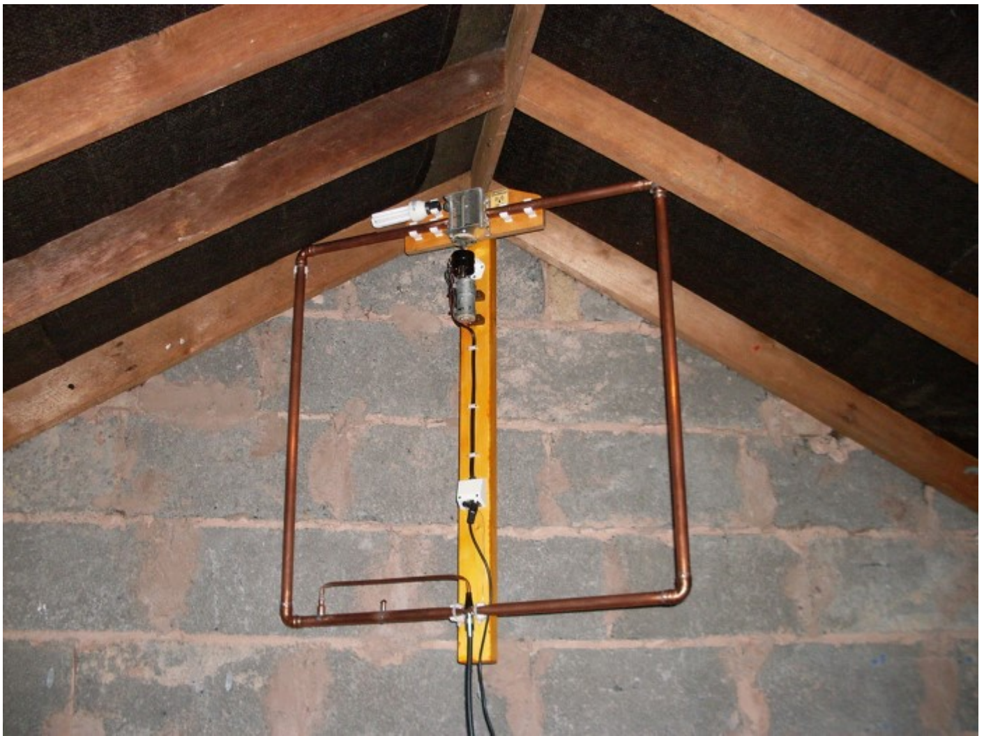
The Mag Loop's final resting place, in the loft, it is supported by just two plastic clips
