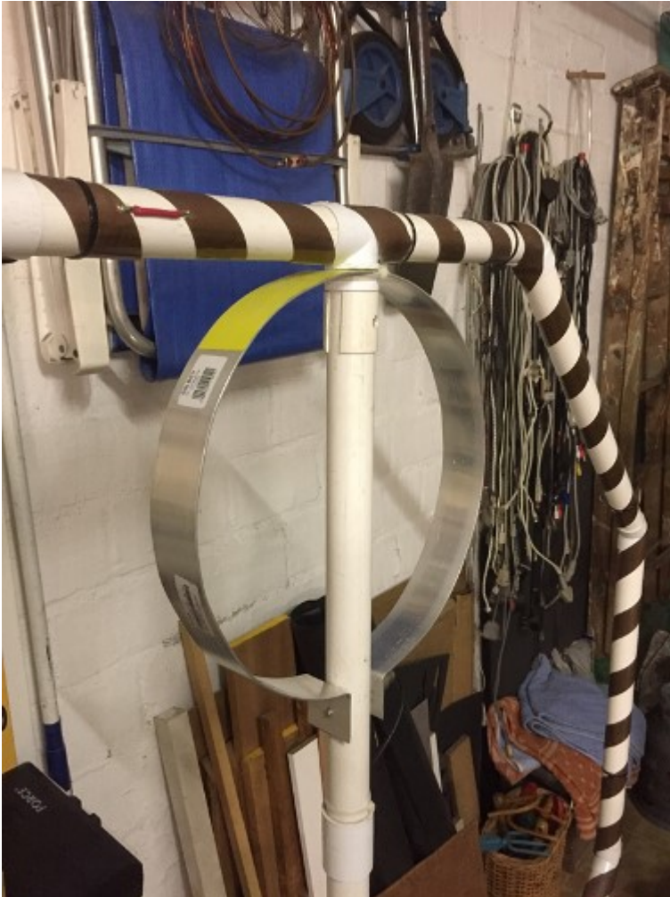
The new coupling loop
