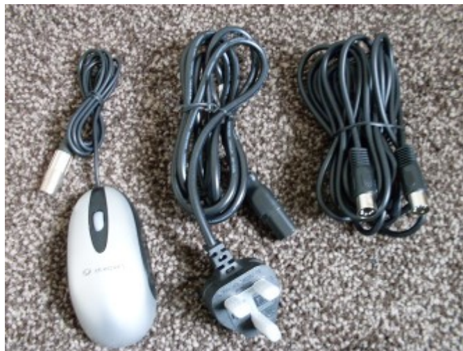
Here are the connecting leads required from left to right, mouse with 5 pin Din plug fitted, IEC mains lead and 5 metre long Din lead.
